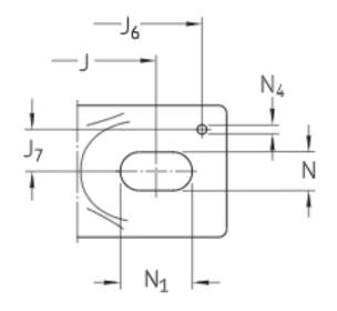
$^{\mathrm{S}}_{\mathrm{1}}$  39.7 mm Distance from locking device side face to raceway centre
